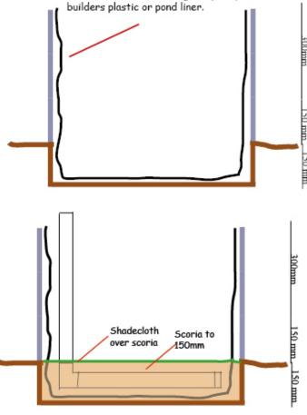
Step Three: Whack up the sides, so the bed has a total depth of 600mm
