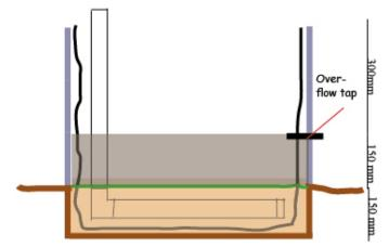
Step Five: Add 150mm of water retentive soil to bed. This is NOT ythe planting area. Add a water tank tap outlet to act as an overflow at 300mm by drilling and attaching to end of bed.
