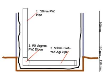
Step Three: Install a length of 50mm pipe (1), a 90degree PVC corner (2) and a length of 50mm slotted agi pipe that will run the length of the bed, along the centre. Place a cap on the end of the agi pipe
