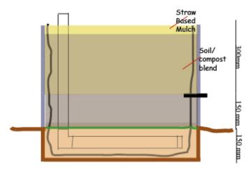
Step Six: Fill the remainder of the bed (another 300mm or so) with a good quality soil/compost blend. Mulch well with a straw based mulch (to about 5-7cm), taking care not to cover the PVC pipe opening.
